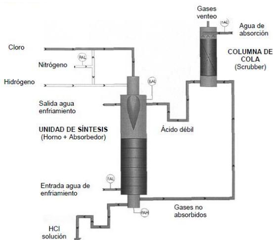
Approximate layout of sodium HCl plant
